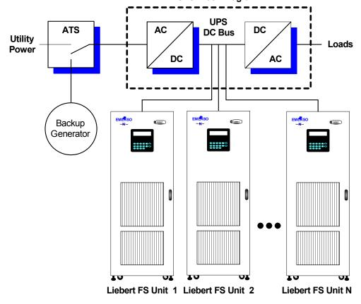
Figure 4 One or more Liebert FS units in parallel with one or more battery strings, battery cabinets or batteries in racks
